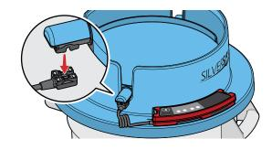
3. Remove the Control Box by gently pulling back the left Snap Clip while lifting the Control Box from the left.
